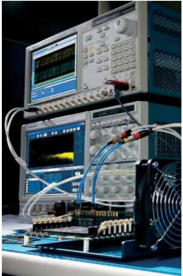
Figure 1. Most measurements require a solution made up of a signal generator paired with an acquisition instrument. Triggering connectivity simplifies capturing of the DUT output signal.
