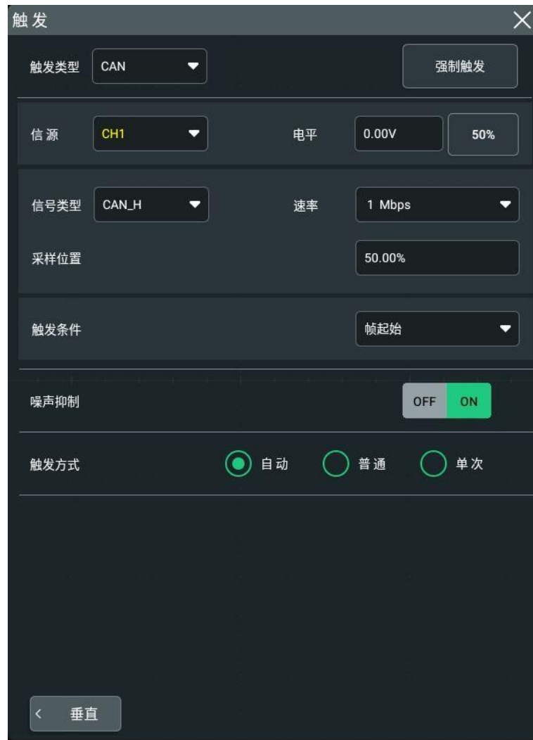
图 8.33 CAN 触发配置菜单
