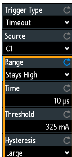
Figure 5-9: Timeout trigger menu
