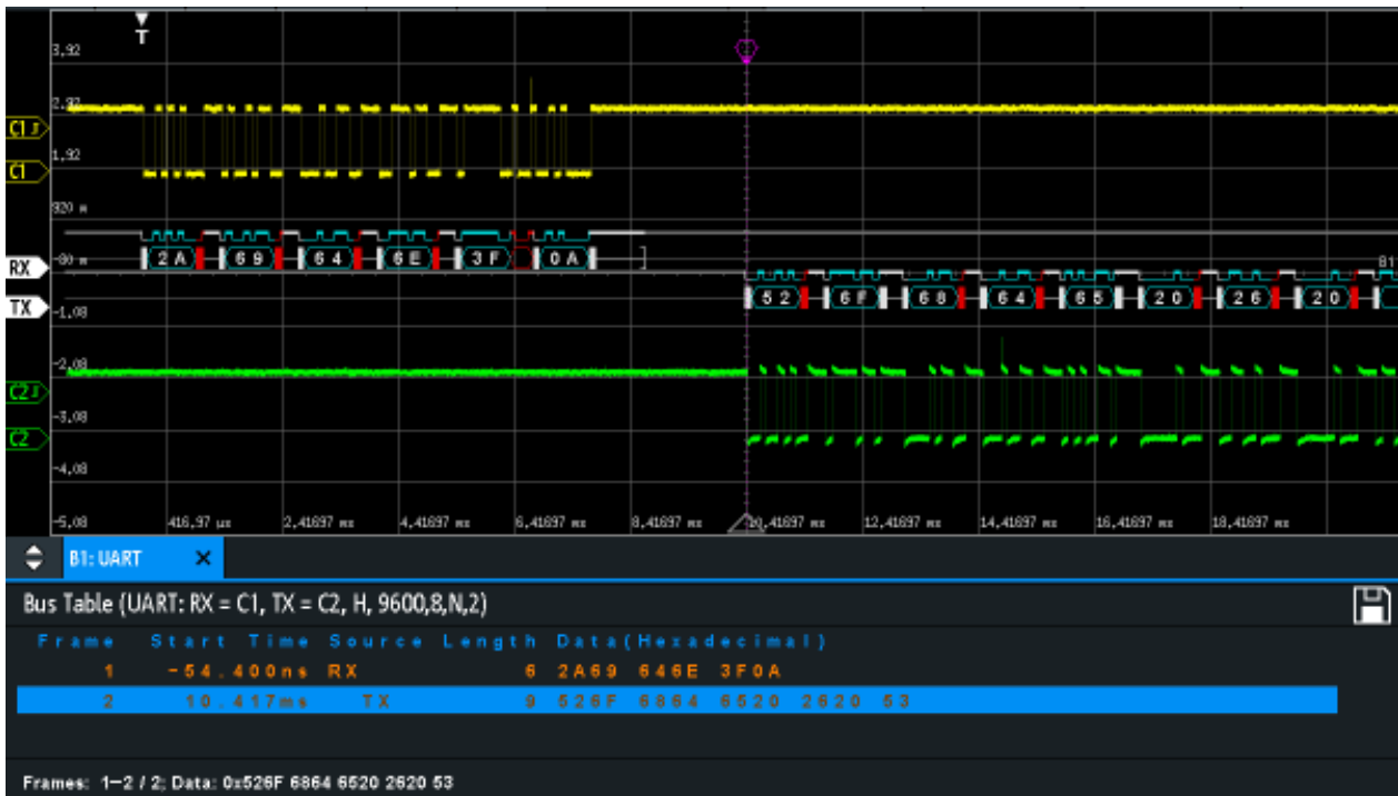
Figure 12-20: Decoded UART signal
