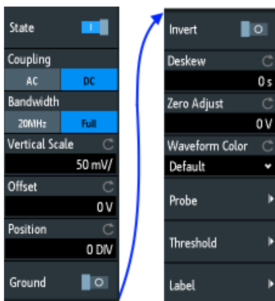
Figure 4-2: Channel menu, split into two halves
