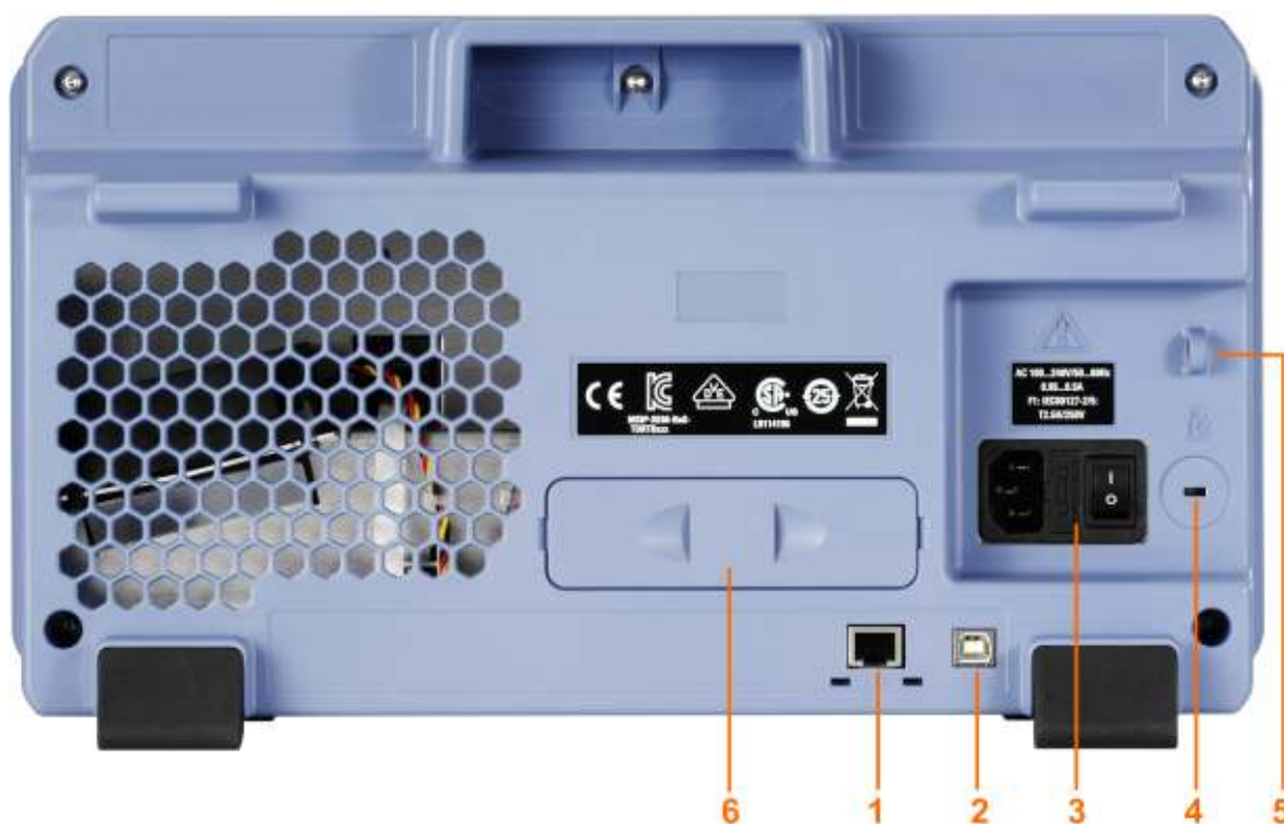
Figure 2-2: Rear panel view of R&S RTB2000
