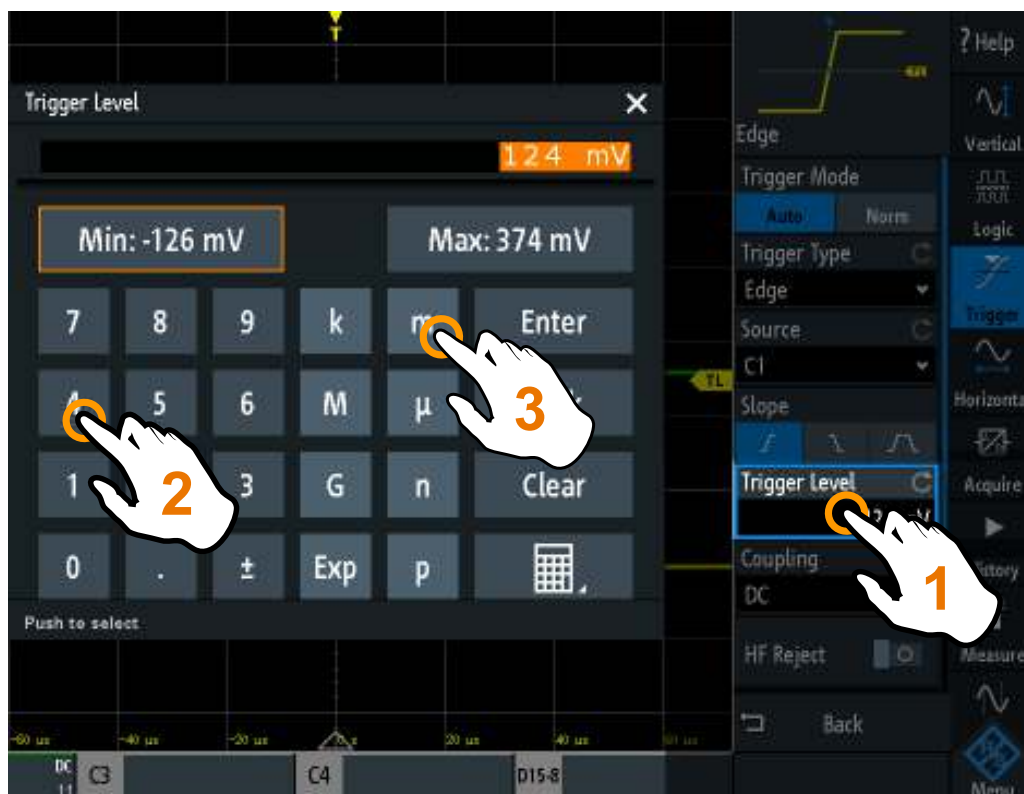
Figure 3-5: Enter numerical value and unit
