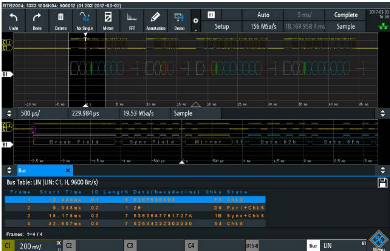
Figure 12-37: Decoded LIN signal with frame table and applied label list
