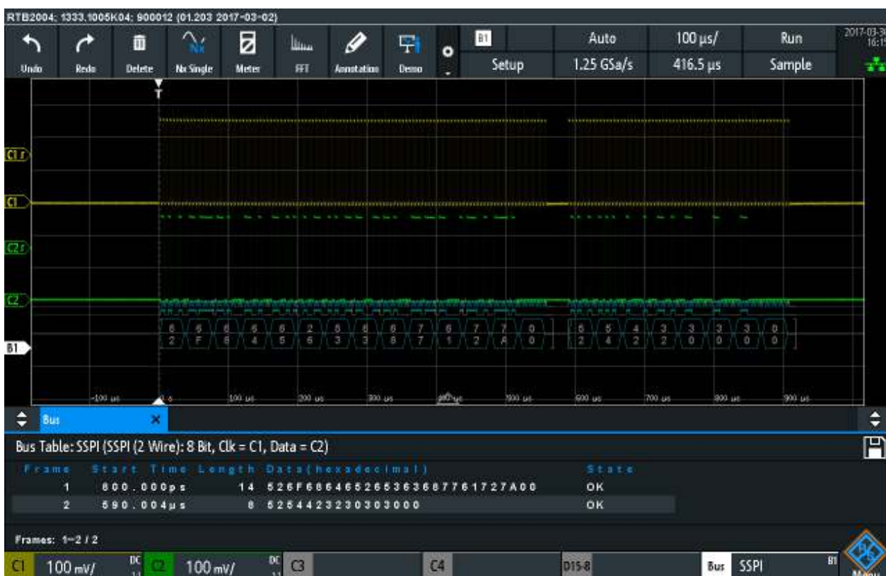
Figure 12-8: Decoded SPI (no CS) signal with Bus Table. The first frame has fourteen words and the second eight words.
