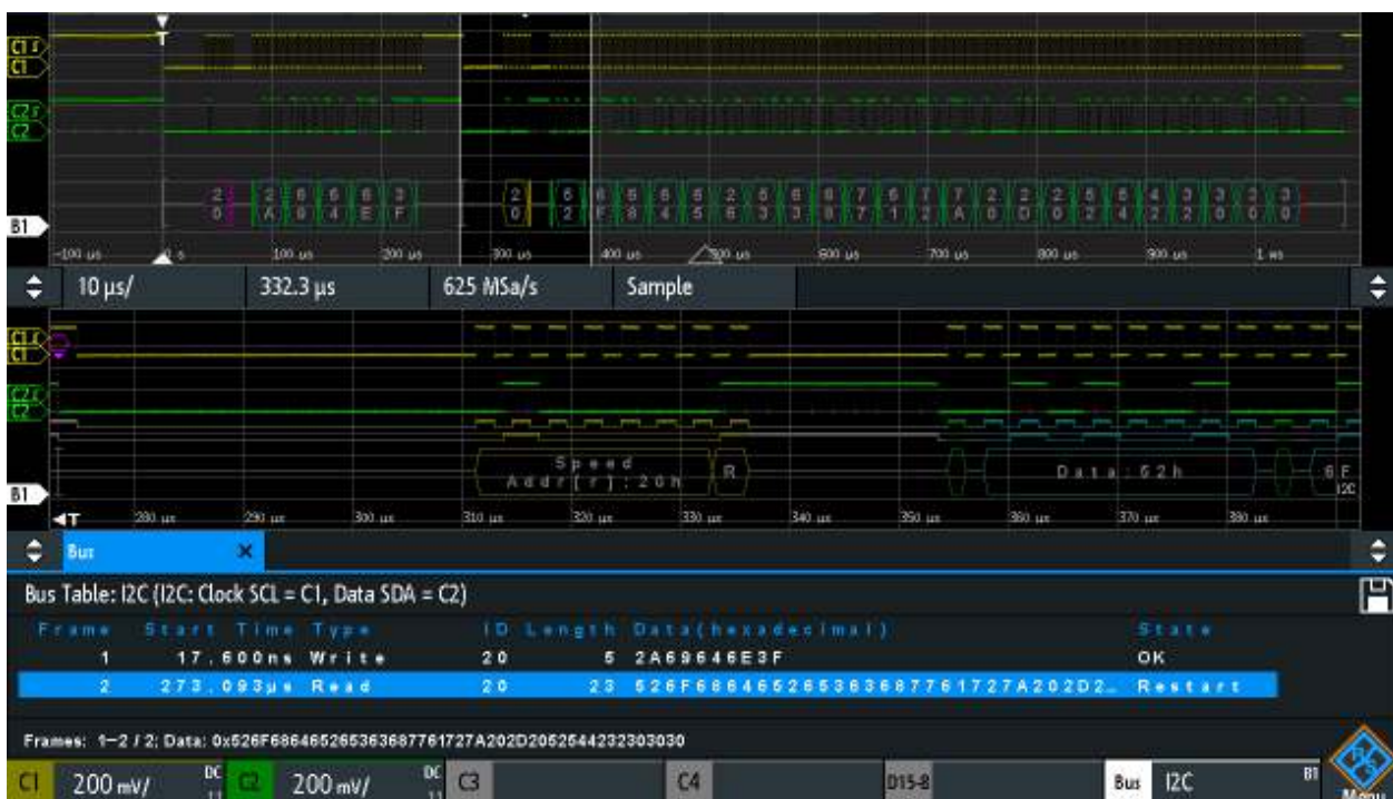
Figure 12-16: Decoded I2C signal with applied label list and zoom on second frame
