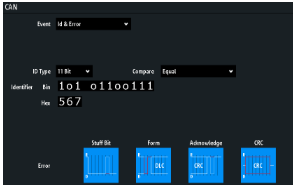
Figure 12-26: Settings for search on CAN bus for frames with identifier 567 (hex) that have an error
