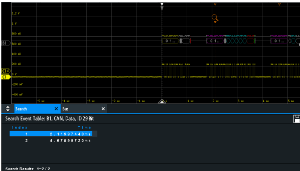
Figure 12-25: Search on a CAN bus for data frames with 29-bit ID
